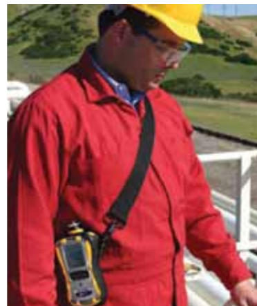
MultiRAE used for worker exposure monitoring at an oil refinery
